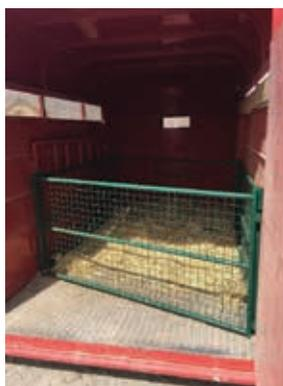
(R): Bedded trailer with partitions. This is an effective way to limit space in the trailer if you have more space than you need. This will prevent pigs from sliding around in the trailer during transport.
